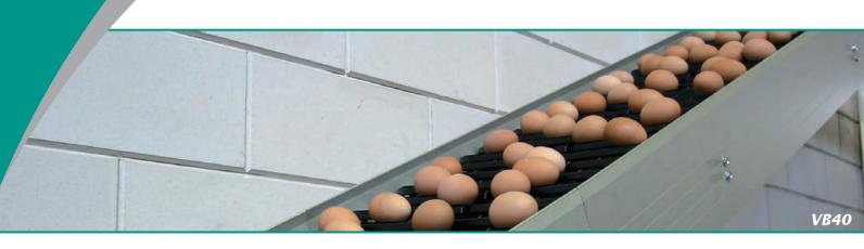
Using the Vencobelt, eggs from different nest rows or houses can be transported to a central collection area. The conveyor system is designed for gentle handling of both hatching and table eggs. With its durable plastic egg carriers and one-chain system Vencobelt can easily be adapted to all circumstances. The design of the carriers and the smooth connections allow a conveyor slope of up to 35 degrees and corners up to 180 degrees.
